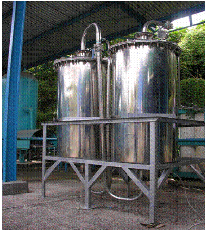
Gambar 12. Adsorber mercury removal skala pilot
